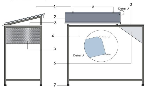
8mm Frosted Toughned Glass with 12mm White Muliti-Wood / WPC base and Triangular Gl Storage fixed on existing drafting table frames
